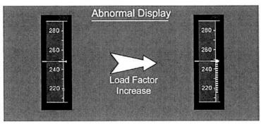
Blocked AOA probes do not affect the current speed indication on the PFD. In addition, in OP CLB or CLB with blocked AOA probes, the pitch order of the flight guidance may be affected by the value of the blocked AOA probes. Therefore, the aircraft may not be able to accelerate in order to reach the target speed.
